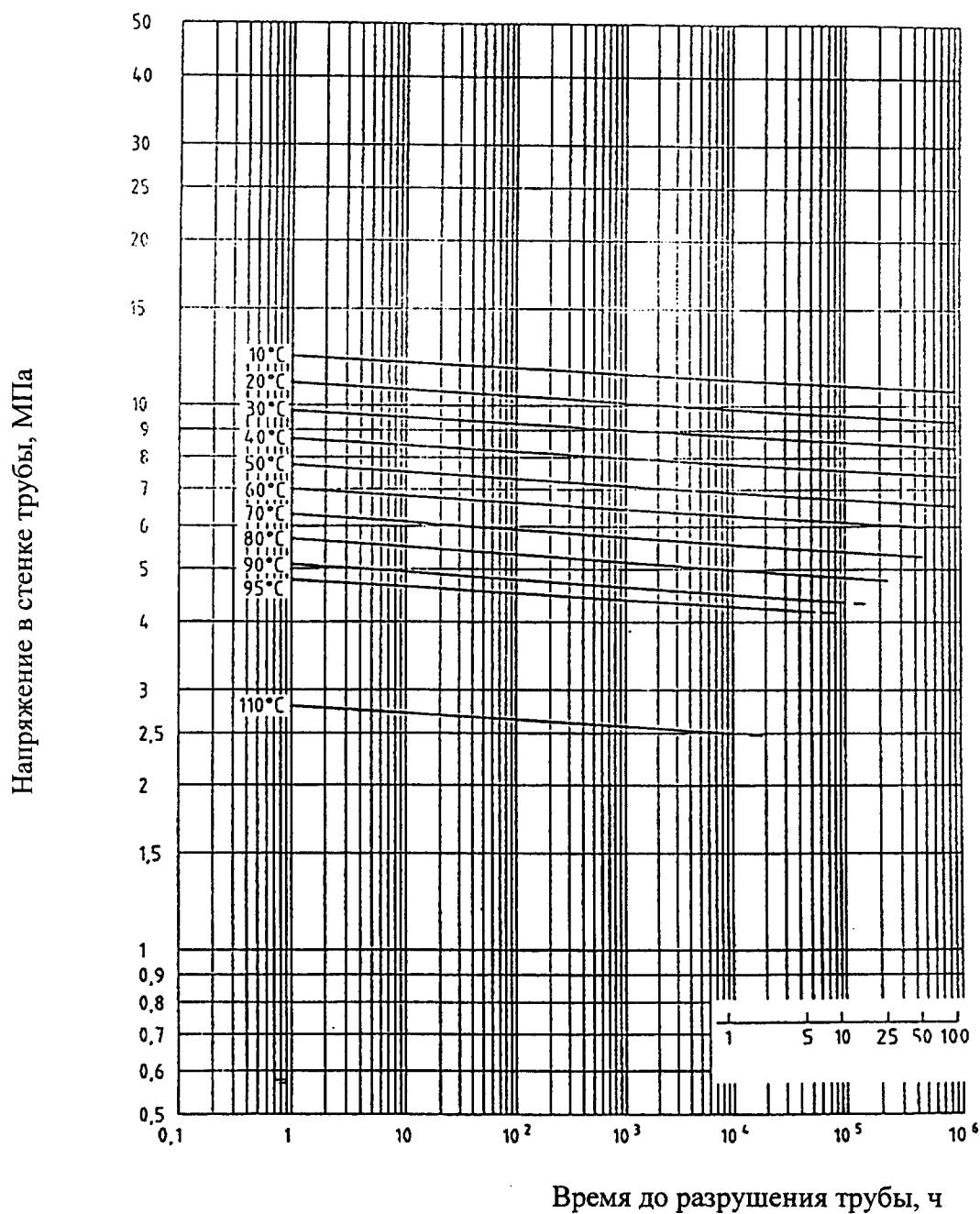
$$\lg(t) = -105,8618 - (18506,15/T) \cdot \lg(\sigma) + 57895,49/T + 24,7997 \cdot \lg(\sigma),$$
